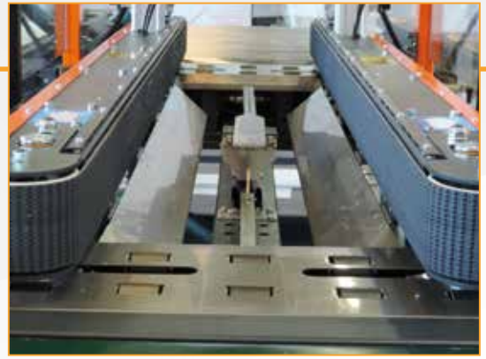
Folding system of bottom flaps (only HM11-TB)
